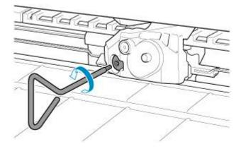
**6.** Remove cutter blade while holding A.
