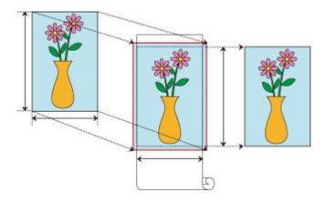
Procedure for printing borderless (without white margins around the edges) by enlarging/reducing documents to match paper size.
