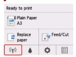
If a different network icon is displayed on the HOME screen, follow the procedure below to enable Wi-Fi connection.
