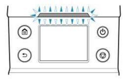
If the **Status** lamp is flashing orange, check the message on the operation panel and take action as necessary.
