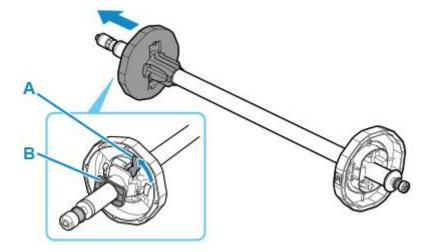
**2.** If using 3-inch core paper, align 3-inch paper core attachment tabs (A) with roll holder holes (B) and insert firmly.
