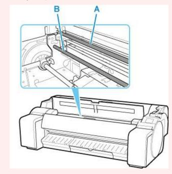
If the paper from a roll is jammed by the paper feed slot
