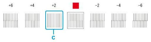
**8.** Open top cover and move angle adjustment lever to match number (or square) of straightest set of lines.
