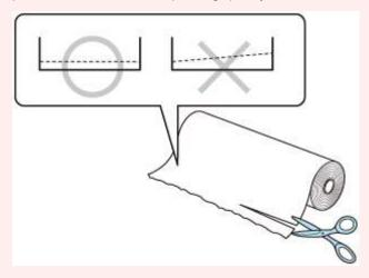
• Align the edges of the paper on both ends of the roll. This may cause feeding problems.
